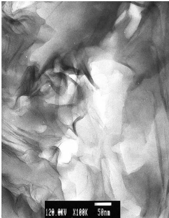
Fig. 3. TEM micrographs of 3 wt% PLSNs. Silicate platelets are visible as grey areas.
